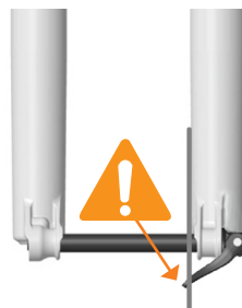
INCORRECTLY INSTALLED AXLE
