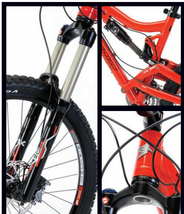
Meaty build: The 6-inch-travel RockShox Lyrik fork. APP suspension links. The Butcher's tapered head tube.
